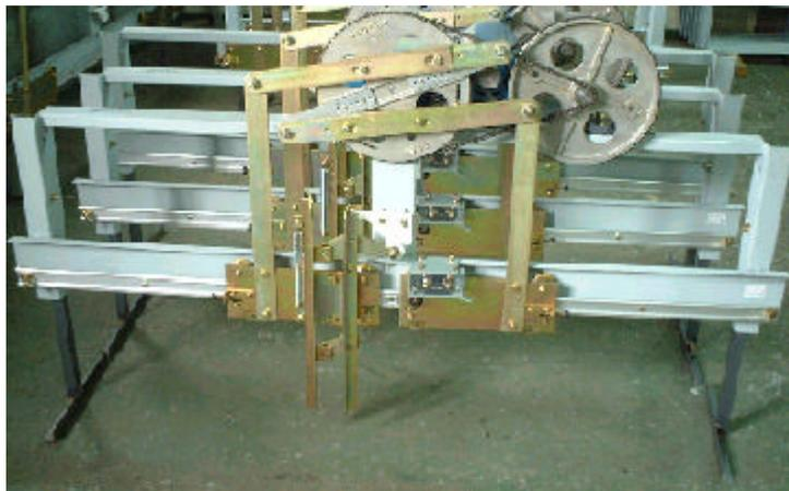
**Figure 1. Door Operator and Car Door**
