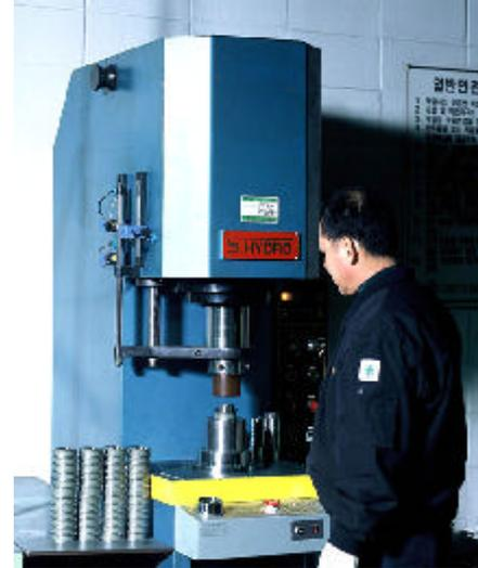
Oil-Pressure Press for Bearing Insertion
