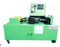
Reliability Testing Apparatus for Escalator Step roller, Guide roller and Parking system roller
