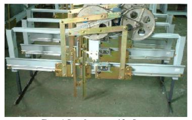
Figure 1, Door Operator and Car Door
