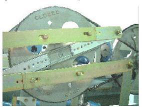
Figure 3, Drive Pulley and Crank Arm
