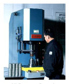
Oil-Pressure Press for Bearing Insertion
