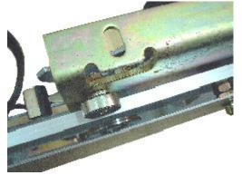
Once moving back the pick-up roller from keeper bolted on the plate of a contact box, it is more definitely what feature they look. And to the right on the top, the fittings are fastened to the hanger plate
