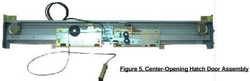
This picture shows the different versions of hatch door from other side. The contact parts and cover are fastened to hanger tract and its lead cables are bolted to connect with power supply. The end tips of hanger plate, slightly seen down describe how it could be installed the door panels. To be more specific there is hanger rollers and upthrust rollers behind hanger plate. In such a way it is possible to lock the hanger plate into the tract.
